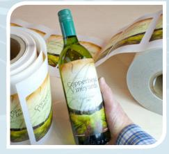
Roll to roll labels, laminated, contour cut with matrix removed and slit into individual rolls ready for application.
