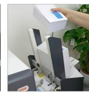
The new ultra-high capacity envelope hopper enables up to 1000 envelopes to be loaded - from the top - enabling continual feeding and printing.
