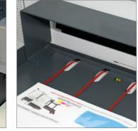
The new light shield helps maintain an improved lighting environment from which the envelope presence sensor beam recognises the presence of the next envelope
