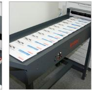
The variable speed shingling conveyor provides an adjustable/ variable overlap of envelopes for quick inspection and easy repacking
