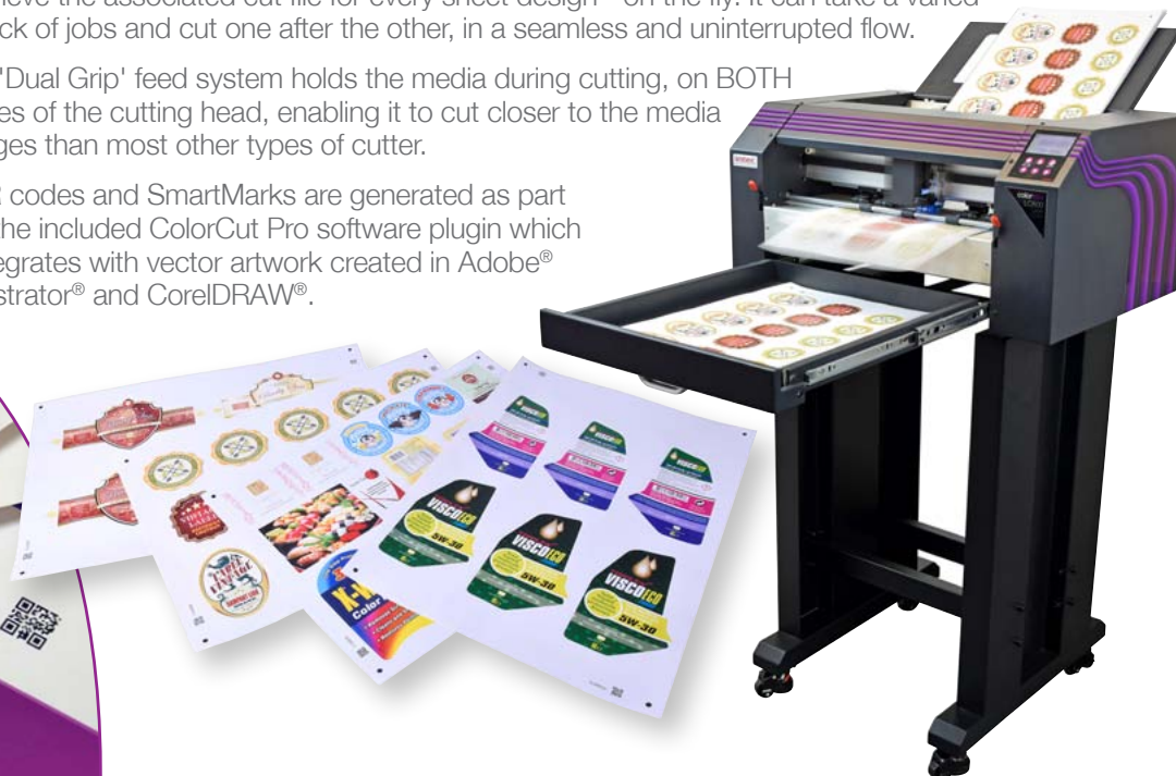
Unique QR codes and Job Numbers applied to each job, enables mixed jobs to be read and cut
