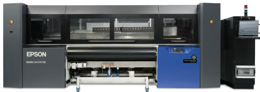
Monna Lisa Evo Tre is an industrial digital textile printer based on Total Solution, the fully integrated system where all components belong to the same process to guarantee the best printing results and the utmost customer satisfaction. This is the result of the synergy of Epson inkjet printing technology with engineering by F.Ili Robustelli and pre/post-treatment and inks by For.Tex, both companies now part of the Epson Group.
